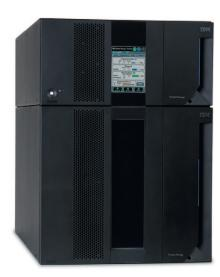
Each model E9U contains 92 physical LTO Ultrium cartridge storage cells and space for up to four LTO Ultrium 6, 5 and 4 tape drives. Additionally, the E9U has space for up to two power supply modules, one of which is redundant. At least one power supply module must be installed if a drive is present in the E9U.
