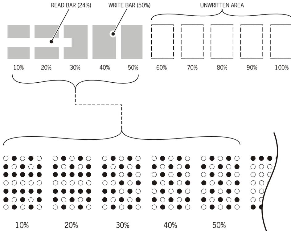
**Note:** The tape bar gets its information from the media information region (MIR) on the tape. The MIR is written to the tape when the tape is unloaded. If the MIR is bad, the tape bar does not display. To rebuild the MIR, see [“Build MIR” on page 4-9](#).
