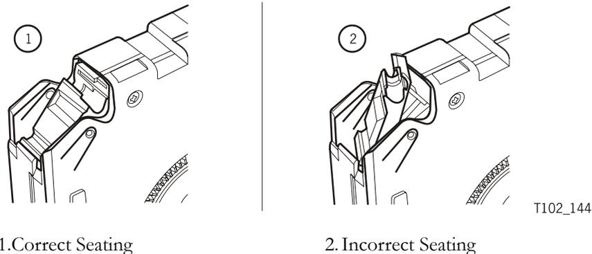
3. Manually insert the tape cartridge into the drive loading slot in the direction shown in [Figure 4-1](#) on page 4-5.
