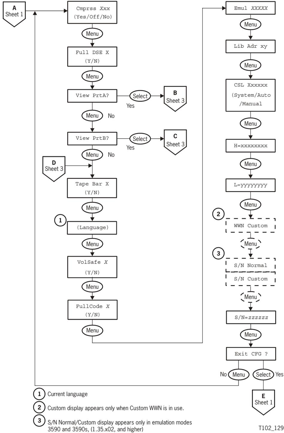
Figure 3-3. Menu Tree—View Fibre Channel Configuration (Sheet 3 of 3)
